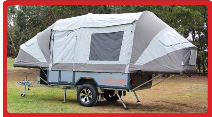
The tent on the Opus is made from a heavy-duty, 400gsm mico-weave poly/cotton blend canvas that combines the high breathability and water-tightness of cotton with the strength and water resistance of polyester. When erect, the tent helps to create the Opus's high ceiling effect that gives you heaps of functional living space inside.
