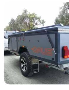
With the inclusion of a rugged, five-leaf off-road suspension and electric disc brakes, with off-road magnets. The Opus has been engineered from the bottom up for true blue Aussie action and adventure. The Opus cruises on 15in, five-stud alloy wheels and all-terrain tyres so it can be trusted to perform even over tough tracks and heavily corrugated roads.
