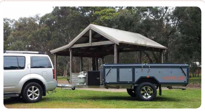
Your chassis on the Opus is hot-dip galvanised to effectively seal it with a super-tough coating designed to resist corrosion and rust. The extended drawbar is made from 100mm x 50mm sections of steel and is fitted with dedicated holders for two jerry cans, a lockable holder for carrying one 9kg gas bottle and a front-mounted toolbox perfect for packing along extra camp gear.
