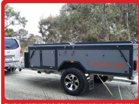
The robust, yet lightweight body of the Opus camper trailer is largely attributed to its composite sandwich panel construction. These dynamic sandwich panel walls are comprised of alternating layers of aluminium and ply with an insulated core to deliver top-notch structural rigidity and a resistance to impact and harsh weather.
