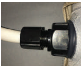
To OPEN valve turn counter clockwise. To CLOSE valve turn clockwise until firm.
